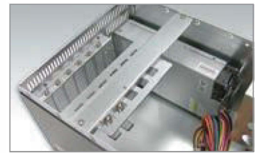
Dual Card Retainers It has two positions for card clamps to hold both PCI and ISA cards tightly
