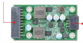
12V / Mini-Fit 8 pin input power connector
