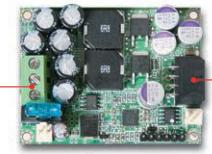
12V / Mini-Fit 8 pin output power connector
