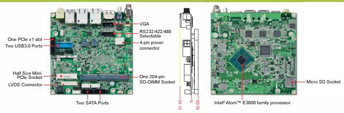
NANO-6060 build with Intel® Atom™ processor E3800 family that not only outputs under 10W for fan-less applications, but also supports a wide industrial temperature from -40°C to 85°C. With its superior up to Quad Core processing power and high capability. Portwell have taken advantage of such technology to furnish a series of products that can meet multiple industrial requirements such as fanless, cost-effective of CPU performance or compact systems..
