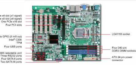
On the basis of Intel® C206 Chipset, RUBY-D711VG2AR supports the latest quad-core 2nd Generation Intel® Core™ i3 and Xeon® processors and provides numerous I/O connectors and also applies high performance in such areas as factory automation, medical, gaming, digital signage, surveillance security monitoring and kiosk.
