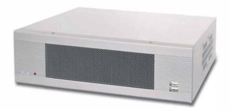
The WADE-2232Q is a rugged and stylish barebones system suitable for embedded applications that stand alone or are rackmounted. Its effective ventilation is achieved by the mesh design of the front panel. No actual tool is needed to release
