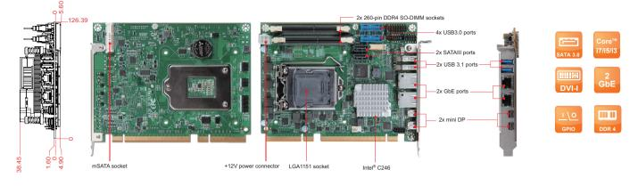
ROBO-6912VG2AR is based on Intel® C246 chipset to support both  $\mathsf{Intel}^{\scriptscriptstyle{(\! 8 \!)}}$   $\mathsf{Xeon}^{\scriptscriptstyle{(\! 8 \!)}}$  and Core<sup>™</sup> i3/i5/i7 processors. Built with flexible PCI express expansions, ROBO-6912VG2AR is suitable for Medical, Industrial automation, and Digital Signage application.
