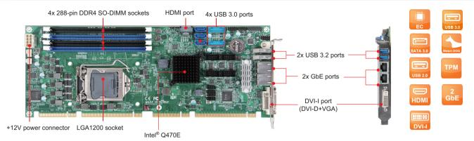
ROBO-8115VG2AR-Q470E is based on Intel® Q470E chipset and workstation processors. Built with flexible PCI express expansions, ROBO-8115VG2AR-Q470E is suitable for Medical, Industrial automation, and Digital Signage application.
