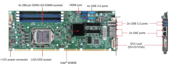
ROBO-8115VG2AR is based on Intel® W480E chipset and workstation processors. Built with flexible PCI express expansions, ROBO-8115VG2AR is suitable for Medical, Industrial automation, and Digital Signage application.
