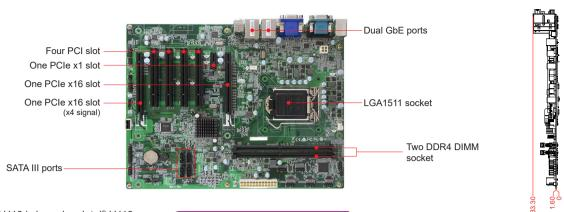
RUBY-D810-H110 is based on Intel® H110 chipset and desktop processor SKU like Intel® 7<sup>th</sup> and 6<sup>th</sup> Gen Core™ i3, i5 and i7 Processors. Built with PCI and PCIe expansions, it's suitable for Medical, Industrial automation, and Digital Signage application.
