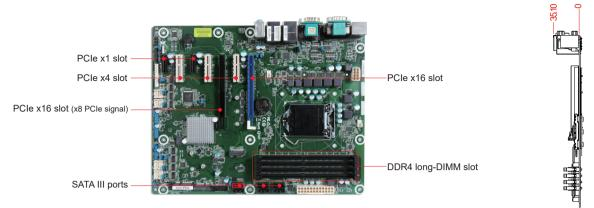
RUBY-D811-Q370 is based on Intel® Q370 chipset and Desktop processors including Intel® 8th/9th Gen Core™ i3/i5/i7 SKU. This board supports DDR4, PCIe 3.0, and SATA III. Those features help you to build high performance and stabile system.
