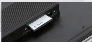
Removable HDD tray and CF cover for easy installation and maintenance.
