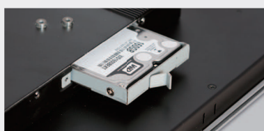
Removable HDD tray and CF cover for easy installation and maintenance.
