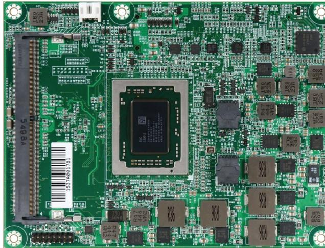
Portwell MEDM-B601 is designed with AMD Quad Core R-Series SoC solution called APU which offers higher computing power and advanced graphic processing ability at lower TDP by introducing AMD 2nd generation heterogeneous system architecture(HSA) for the medical healthcare systems.
