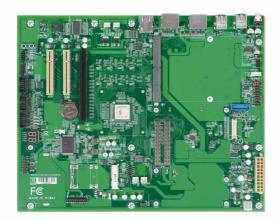
MEDM-C600 ATX carrier board is development platforms that enable medical customers to begin development on an application specific design with Portwell COM Express module quickly and easily. The MEDM-C600 provides a wide range connectivity for prototype and development ease and flexibility.
