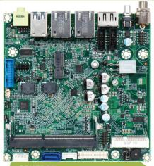
NANO-6062 build with Intel® Atom™ processor E3900 series. Not only does it operates with TDP under 12W for fan-less applications, but it also supports industrial temperature range from -40°C to 85°C and wide voltage of power input from 12V to 24V.
