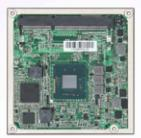
New Mobile based Type VI COM Express module with DDR3L SDRAM, VGA, eDP, HDMI, Gigabit Ethernet and 3Gbps SATA.
