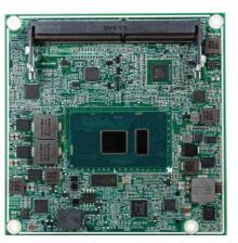
PCOM-B644VG brings three important factors, DDR4 memory support, Gen3 PCIe support, and 30% faster graphic performance. The Gen3 PCIe support provides faster PCIe speed so that the performance of PCIe expansion card will be better. It is crucial for Networking and Medical related applications. The enhanced graphic performance brings 4K support. The OTG support gives customer more flexibilities on developing new applications in different usages.
