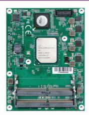
Portwell PCOM-B701 is designed with Intel® new Atom™ processor with brand new Type 7 pin definition. It's built in with 10GbE Ethernet KR interface and DDR4 ECC SO-Dimm support which provide high CPU computing, excellent Ethernet performance. Extend PCIE Gen3 ports in PCOM-B701 can support high speed IO card for more applications. In the meantime, it's compatible with Type 6 carrier.
