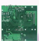
Portwell's 1st COM Express® Rev3.0 Type 7 Carrier which supports four 10GbE optical and fiber phys, NC-SI interface and up to 32 PCI Express lanes.
