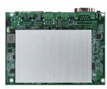
PEB-2773 build with Intel® Atom™ processor E3900 series. Not only does it operates with TDP under 12W for fan-less applications, but it also supports industrial temperature range from -40°C to 85°C and wide voltage of power input from 12V to 24V.
