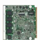
Intel® Atom™ Based Qseven 2.0 module board with memory-down, Dual DP, SATA, PCIE, Gigabit Ethernet and eMMC
