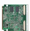
Qseven module based on Freescale™ i.MX6 family, ARM™ Cortex-A9, Solo / Dual / Quad core processor with onboard 1GB DDR3 (up to 2GB), PCIe 1-lane interface, VGA, HDMI, single LVDS 1-ch or dual LVDS (18/24-bit) 2-ch and CAN Bus.
