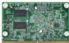
The SMARC ("Smart Mobility ARChitecture"), small form factor of lower power, cost concern, and high performance, is used as building blocks for portable and stationary embedded systems. The SMARC pin-out is optimized for the features common to ARM CPUs and not common to the x86 PC world. The modular approach allows scalability, fast time to market and upgradability while still maintaining cost performance, low power and small physical size.
