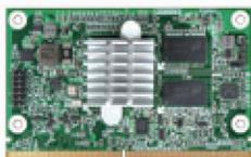
PSMC-M640F is design as CPU module series with SMARC form factor. It is based on embedded Freescale™ i.MX6 processor, an ARM® Cortex®-A9 processor, Single, Dual and Quad-Core.
