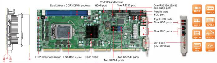
ROBO-8110VG2AR is based upon the Intel® C206 chipset and workstation processor sku like Xeon® and Core™ i3. Built with flexible PCI express expansion, it's suitable for medical, industrial automation, and Digital Signage applications.
