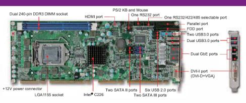
ROBO-8111 VG2AR is based on the Intel® C216 chipset and workstation processor sku. Built with flexible PCI express expansion, it's suitable for medical, Factory Automation, and Digital Signage applications.
