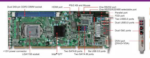
ROBO-8111VG2AR-Q77 is based on Intel® Q77 chipset and Core™ i7/i5 sku processor. It's suitable for Medical, Factory Automation, and Digital Signage applications.
