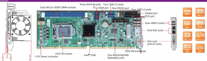
ROBO-8112VG2AR is based on Intel® C226 chipset and workstation processor sku like Xeon® and Core™ i3. Build with flexible PCI express expension, it's suitable for Medical, Industrial automation, and Digital Signage applications.
