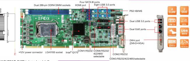
ROBO-8113VG2AR-Q170 is based on Intel® Q170 chipset and desktop processors. Built with flexible PCI express expansions, ROBO-8113VG2AR is suitable for Medical, Industrial automation, and Digital Signage application.
