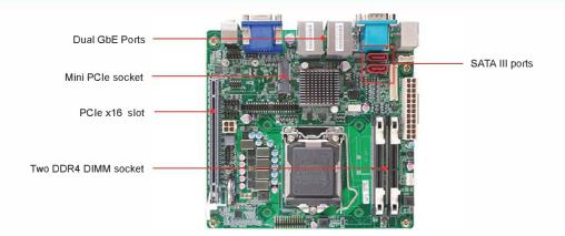
WADE-8210 is based on Intel® H110 chipset and Desktop processors including Intel® 6/7th Gen Core™ i3/i5/i7 SKU. This board supports DDR4, PCIe 3.0, and SATAIII. Those features help you to build high performance and stable system.
